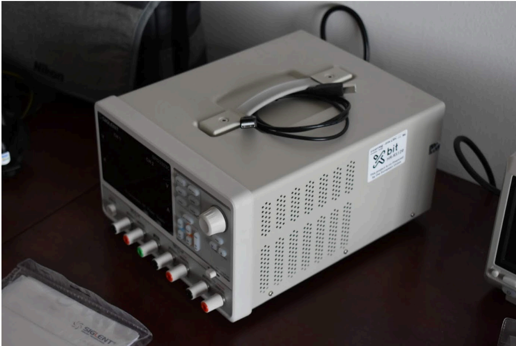
Slika 11. Siglent SPD33 Power supply 220W
